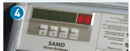
IN CASE OF DETECTION, SAMD GENERATES AN ACOUSTICAL AND A VISUAL RED ALARM
